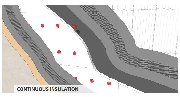
Amvic's EPS is non-structural, rigid insulation boards made from 100% virgin, closed cell, Expanded Polystyrene (EPS). Board are either aged in ambient air for five weeks or kiln-dried.
